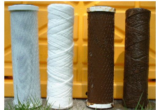
Clean and clogged prefilters
