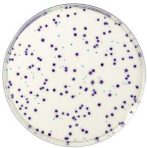
One type of test plate: purple dots are colonies of E. coli ; blue dots are colonies of other coliforms.
